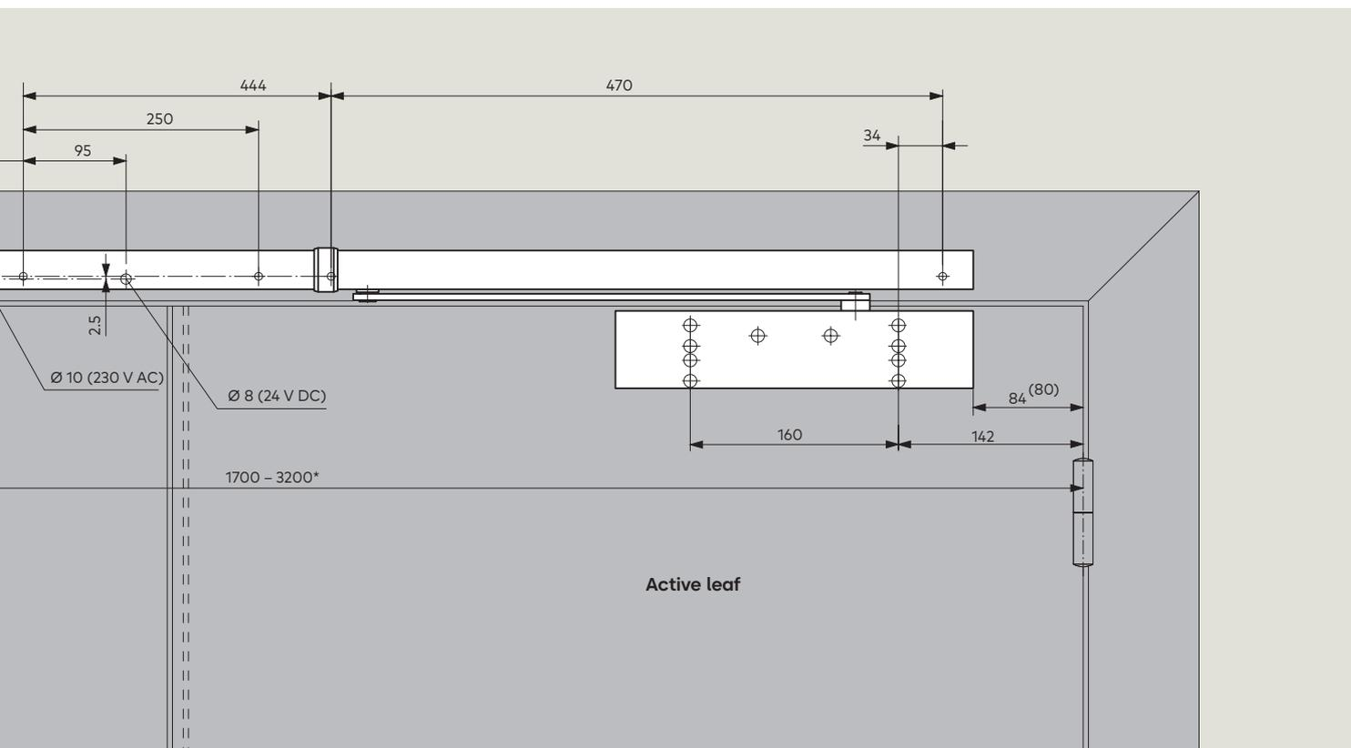
\* In the case of particularly large and heavy doors (over 2500 mm), we recommend that EM hold-open magnets be employed instead of the electro-mechanical hold-open unit.
