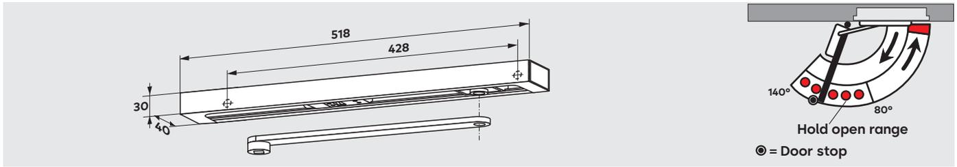
The **G-EMF** slide channel assembly enables the door to be held open securely at a preselected position without fall-back. The hold-open point can be adjusted within an opening angle of approx. 80° and 140°.
