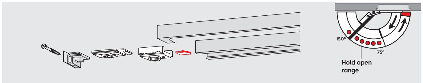
The **RF hold-open unit** enables doors to be securely held without any fall-back at precisely the required position up to an opening angle of approx. 150°. The hold-open function can be easily switched on and off by the user, and the release force can be adjusted to the door type concerned.
