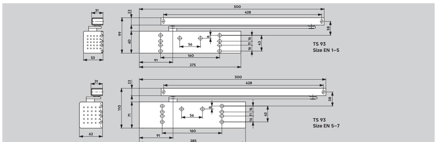
**Standard mounting backplate with universal fixing hole system**
