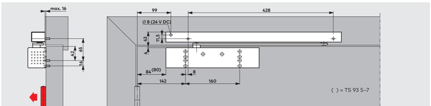
**TS 93 B** closer with G-EMF slide channel assembly, pull-side fixing
