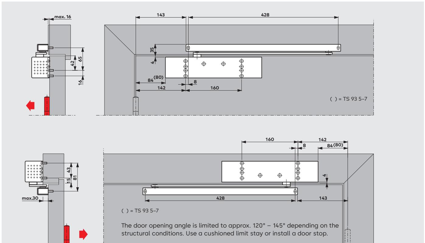
**TS 93 B** door closer with G-N slide channel assembly, door leaf fixing on the pull side and transom fixing on the push side.
