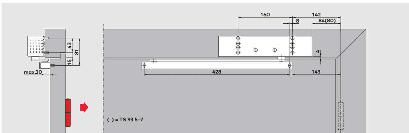
Transom fixing (overhead frame fixing) of the TS 93 B on the push side. Backcheck and delayed action non-operative with this fixing arrangement. The door opening angle is limited to approx. 120° to 145°, depending on the structural conditions. In order to prevent damage to the wall and door, a door stop should be installed to limit the maximum angle of door opening.
