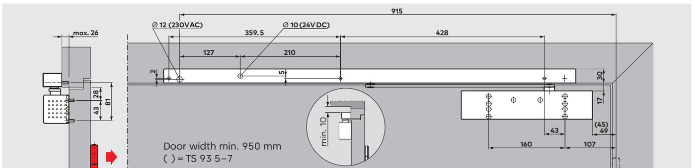
**TS 93 G** door closer with G-EMR slide channel assembly, push-side fixing
