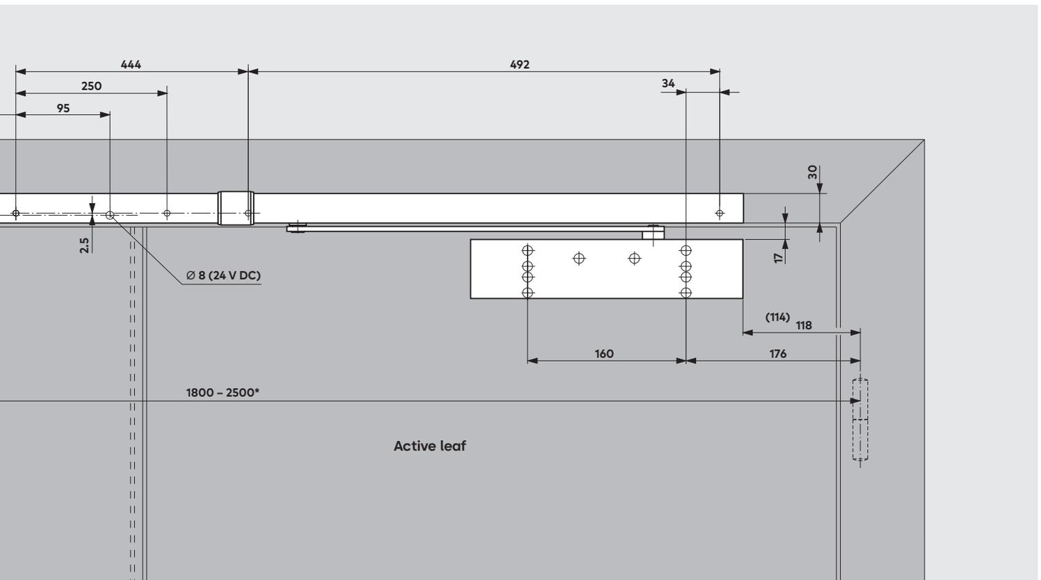
\* In the case of particularly large and heavy doors, we recommend that EM hold-open magnets be employed instead of the electro-mechanical hold-open unit.
