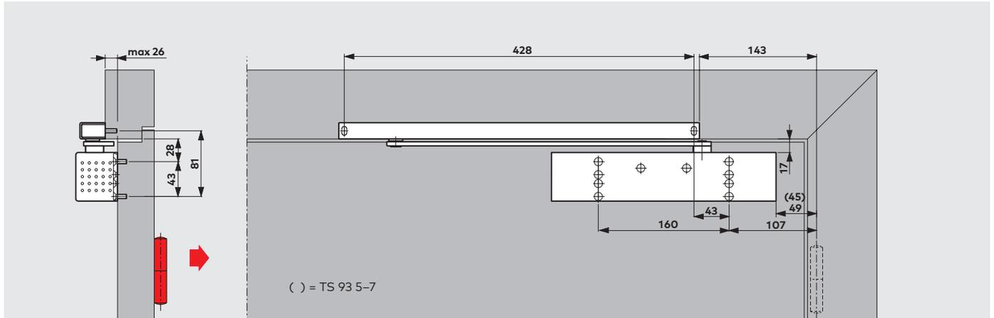
Door leaf fixing (standard installation) of the TS 93 G on the push side.
