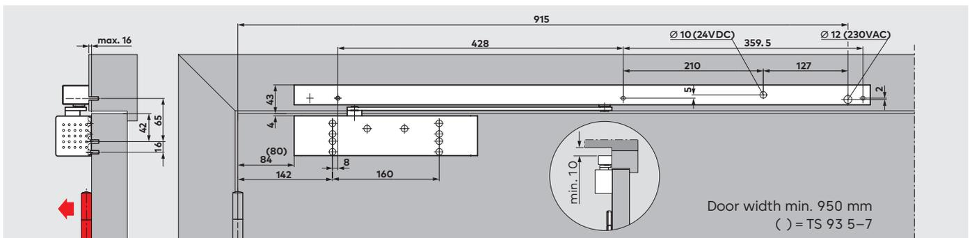
**TS 93 B** closer with G-EMR slide channel assembly, pull-side fixing
