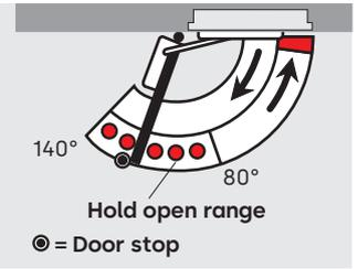
The G-EMR slide channel assembly enables fire and smoke doors to be held open securely at precisely the angle required, and monitored and controlled completely independently of other systems. The hold-open point can be adjusted to opening angles between approx. 80° and 140°.
