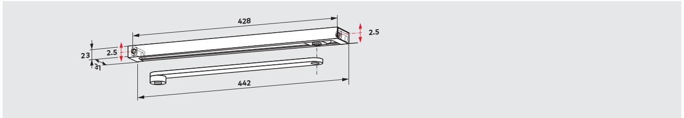
The **G-N slide channel** assembly incorporates the slide arm, slide channel, slide block, fixing adapters, screws and end caps.
