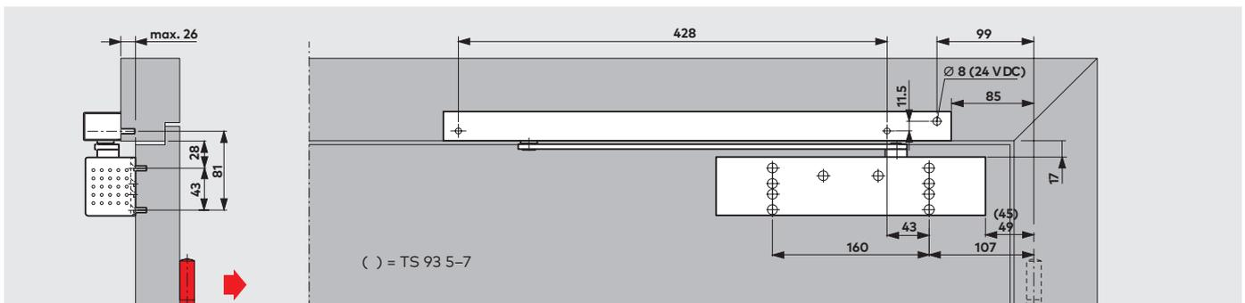
**TS 93 G** closer with G-EMF slide channel assembly, push-side fixing
