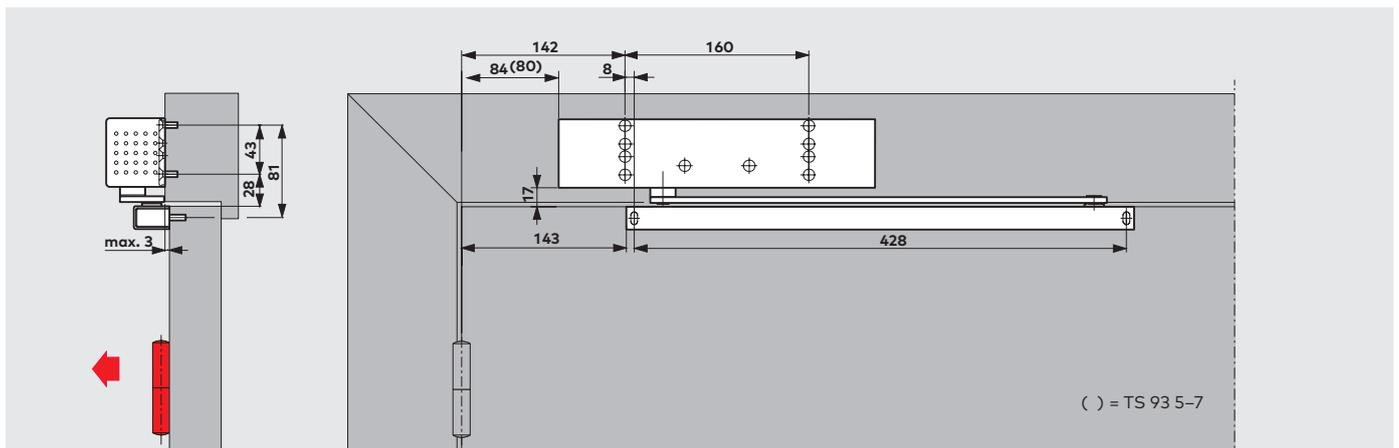
Transom fixing (overhead frame fixing) of the TS 93 G on the pull side.
