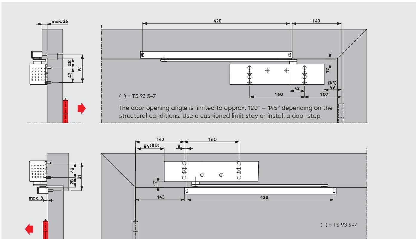
**TS 93 G** door closer with G-N slide channel assembly, door leaf fixing on the push side and transom fixing on the pull side.
