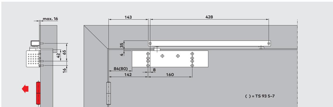
Door leaf fixing (standard arrangement) of the TS 93 B on the pull side.
